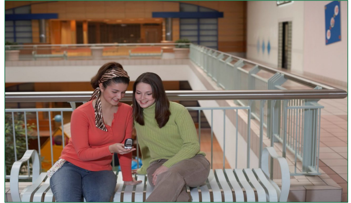
Avoid placing furniture against guardrails. This can be considered an attractive nuisance.
